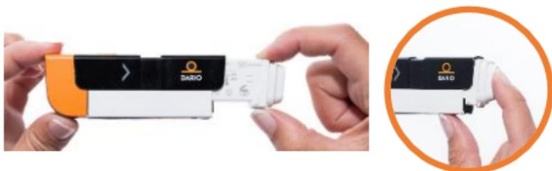
4. Insert the cartridge into the housing until it snaps into place.
