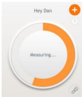
*The glucose test result appears on the screen after six (6) seconds and is automatically saved to memory.*
