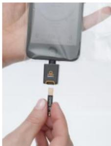
*The Dario App screen instructs you to place a drop of blood on the test strip, as shown in the image below.*
