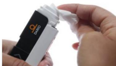
To ensure effective disinfection, let the solution sit on the meter, housing, orange lancet cover, and white cartridge cover for at least two (2) minutes. Allow the meter, housing, orange lancet cover, white cartridge cover and cartridge cap to completely dry before use. Wipe off any remaining residues with a clean, soft, and dry paper cloth.
